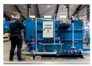
Incineration of waste and oil sludge, to achieve lower operational costs and reduced environmental impact, while experiencing a 15% higher burning capacity compared to similar marine incinerators.
