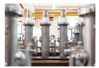
Valves and venting equipment reducing emissions from cargo during voyage and thereby ensuring cost savings, safety for the crew and the environment.
