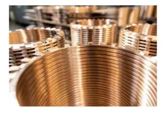
Piston rod stuffing boxes for two-stroke engines continuously improved to live up to new fuel types entering the market. A trusted partner who delivers quality on time and has a sustainable profile.
