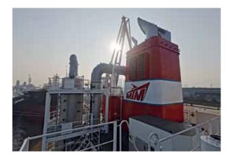
PureteQ is an engineering company that designs and services built-to-fit maritime exhaust gas cleaning systems, also known as scrubbers. PureteQ maritime scrubbers can handle loads of up to 100MW and are equipped with a user-friendly control system allowing real-time remote access and support. The energy performance is superior due to the patented hydrodynamic fluid distribution system, which eliminates interior obstructions.
